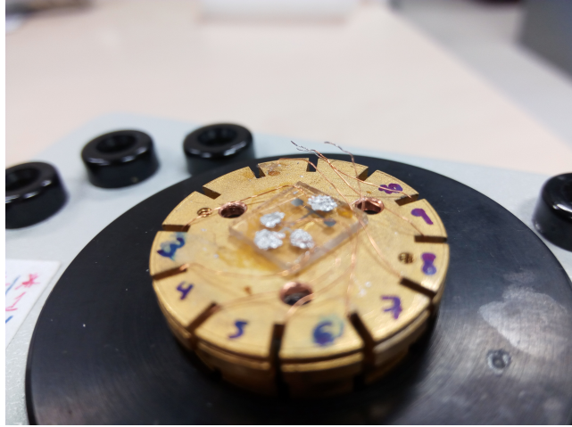
Figure 6: Al/AIO x /Al/EuS/glass structure mounted on the resistivity measurements sample stage of the Quantum Design's PPMS system
