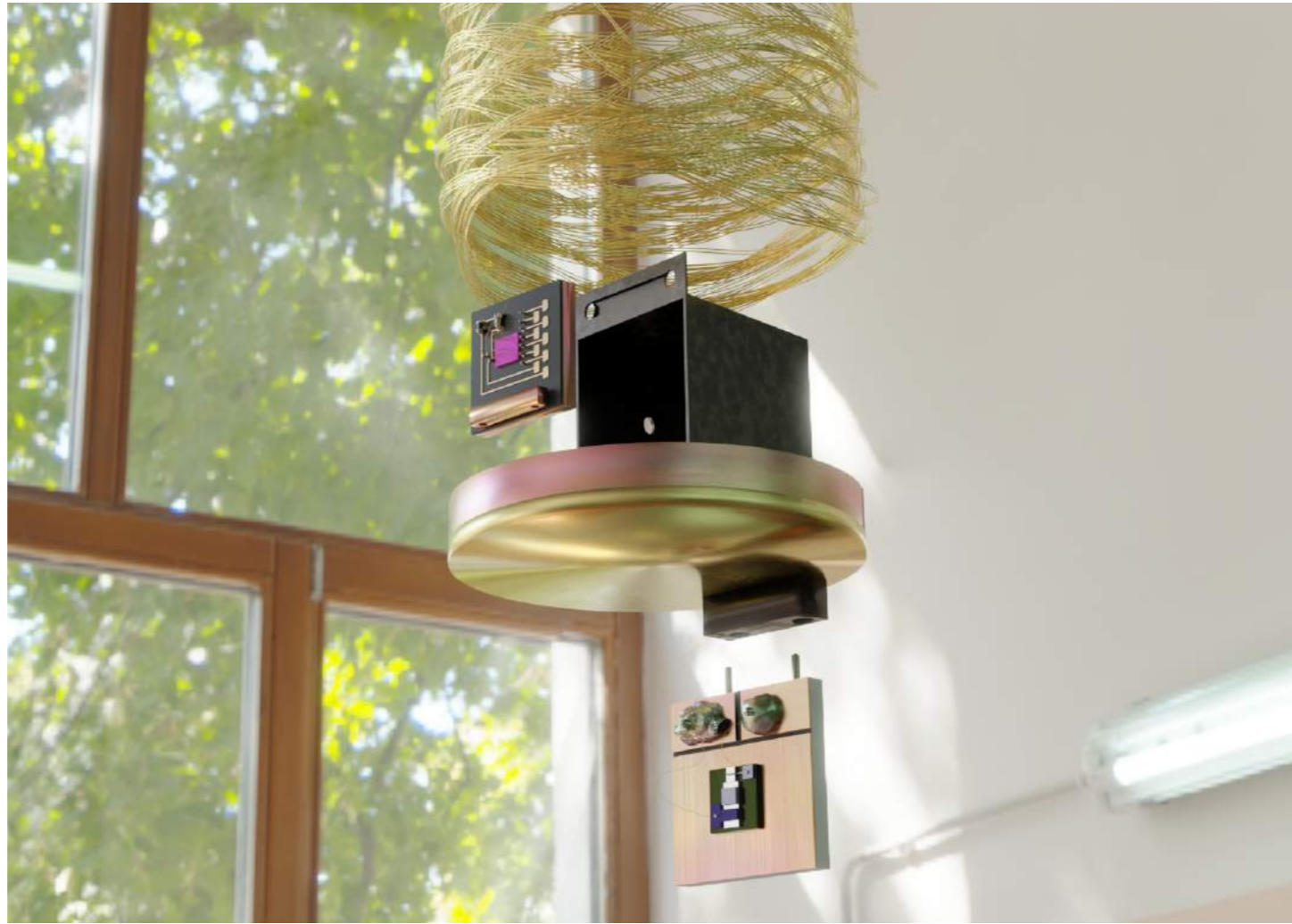
Integration of the sensor and the first stage of read-out: Both devices must be located close to each other, in a zone with the lowest temperature. SQUID read-out must be shielded from the magnetic field applied to the sensor in order to initiate the spin splitting.
