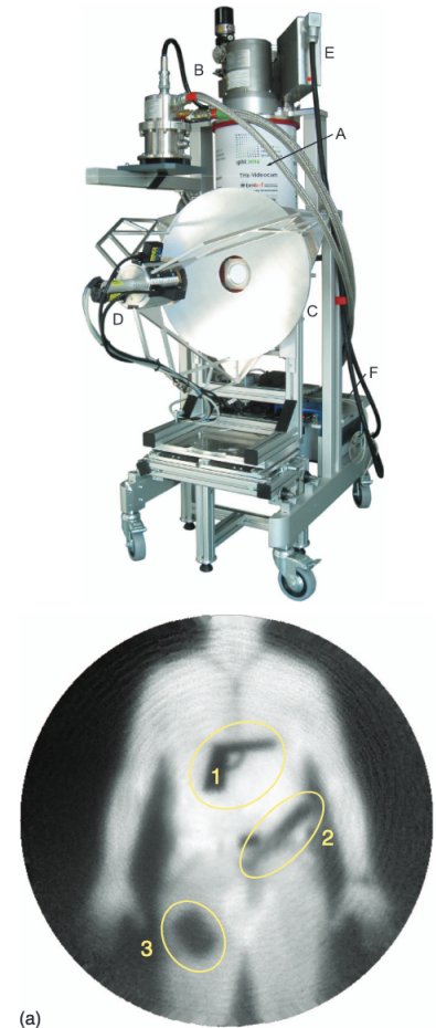
Figure 3.30: Portable system for stand-off surveillance , shown on top image, integrates cryostat with a 20 TES array (A), pulse tube cooler (B), Cassegrain main mirror (C), optomechanical scanner (D), readout electronics (E) and control electronics (F). At bottom image, example of image acquired with the system, of a person carrying concealed objects: a mock-up handgun (1), a plastic tube filled with sugar (2), and a jelly bag (3). Source: (42).
