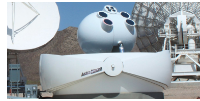
Figure 3.34: Lunar Laser Communication Demonstration - LLCD successfully demonstrated for the first time high-rate duplex laser communications between a satellite in lunar orbit, the Lunar Atmosphere and Dust Environment Explorer (LADEE), and multiple ground stations on the Earth.
