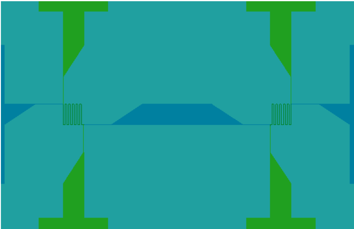
Figure. First proposal, calling for a lithography of the NIS junction. This solution has been considered too risky for the junction itself.
