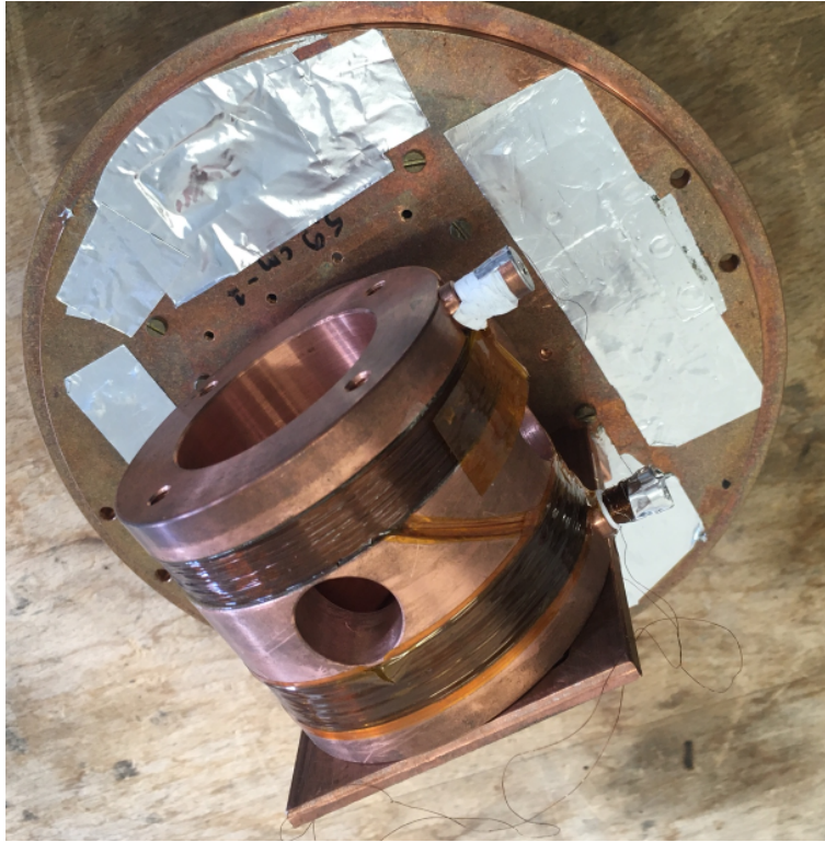
Figure. The fabricated Helmholtz coil, mounted on the 100mK stage of the NIKA0 system. Ready to be integrated into the cryostat. The small hole is where the optical beam is entering.
